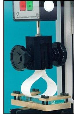
**Significance:** High stickiness indicates, considerable ease of “attaching” to surfaces where detachment is difficult, and ruptures of the facestock material in many cases and can cause bleeding. The opposite holds true for low tack.
